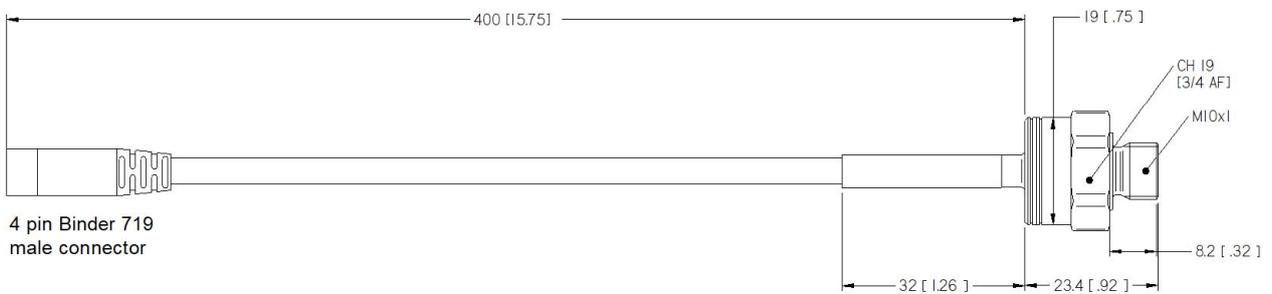
The sensor ends with a 4 pins Binder 719 male connector. The image below shows the connector pinout from solder termination side.
