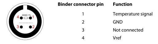
**Please note**: as shown here above a  $2k\Omega$  1% resistor is mounted between pin 1 and pin 4
