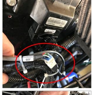
To connect to the on-board gear sensor, plug the 6pins Sumitomo connector to the vehicle harness 6pins black Sumitomo connector (see picture on the right), placed under the front bonnet, near the front right wheel.
