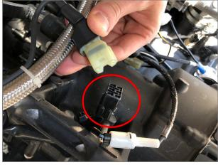
The first analog channel must be used to connect to the on-board gear sensor. The other three MXm analog channels (labelled "CH#") can be used for sensors connection (i.e.: AiM temperature, pressure and position sensors), in order to record additional parameters for driver coaching, chassis analysis and engine monitoring.
