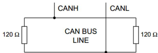
Each end of the CAN bus is terminated with 120Ω resistors in compliance with the standard to minimize signal reflections on the bus. You may need to place a 120Ω resistor between CAN-L and CAN-H.
