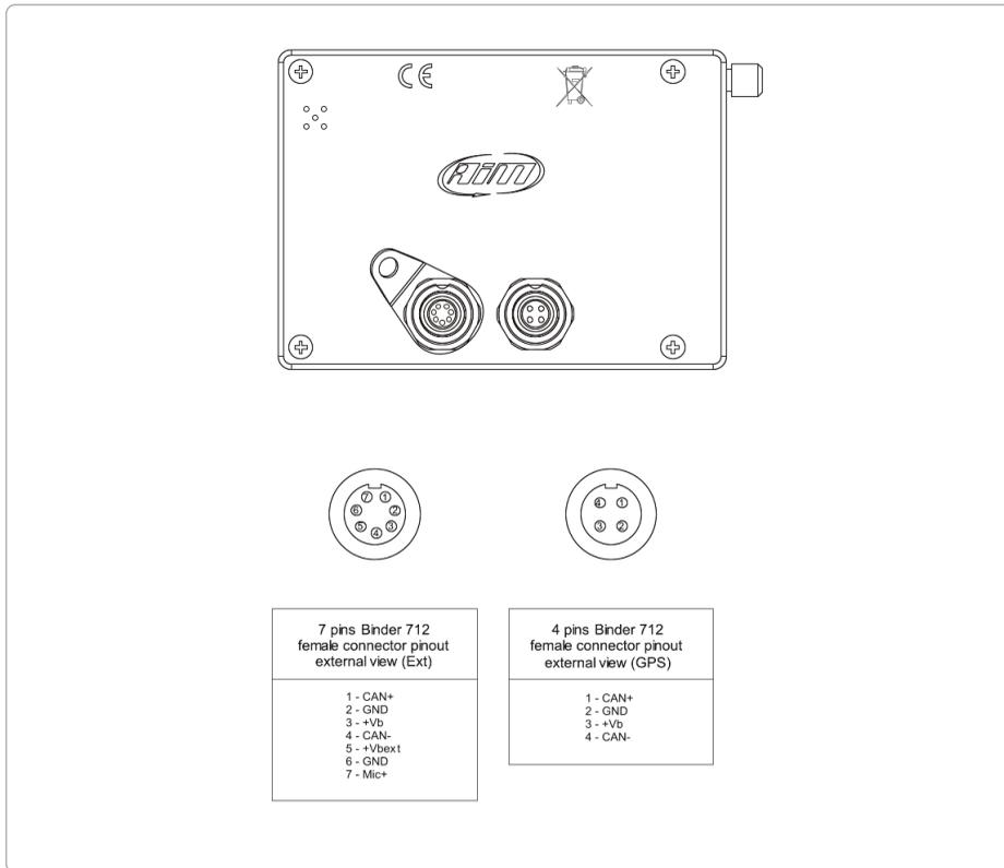
Smartycam GP HD rev. 2.1 pinout
