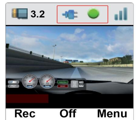
SmartyCam can be switched ON/OFF using the central button. The system asks for confirmation.
